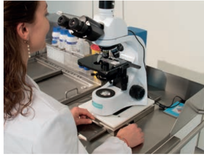
Adjustable microscope sleigh for ergonomic movement forward-backward
