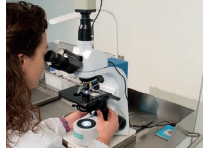
Adjustable microscope sleigh for ergonomic movement forward-backward
